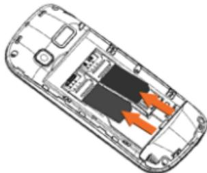
3. Finally, insert the battery and place the rear cover of the mobile phone.
