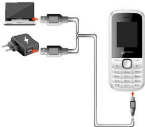
2. Connect the charger to a power socket or connect the USB jack of the cable with your PC or laptop.
