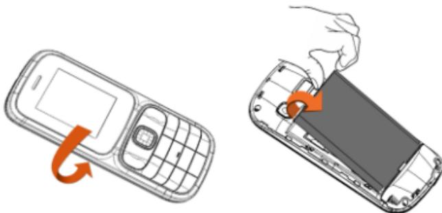
2. Insert the SIM card(s) correctly in the card slot(s), as shown in the following image:
