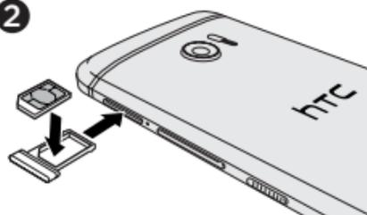
2. Place your nano SIM card into the tray, with the gold contacts facing **up** and cut-off corner facing **out**.
