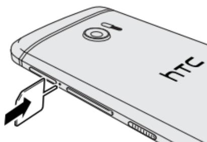
1. With the phone facing **down**, insert the tip of the tray eject tool that came with your phone (or a small bent paperclip) into the nano SIM tray eject hole that's on the left side of your phone.
