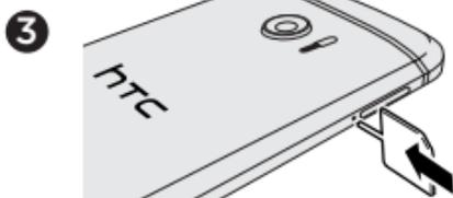
3. Use the same tray eject tool to eject the microSD™ card tray on the other side. Pull the tray out.
