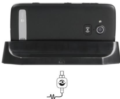
1. Insert the small end
