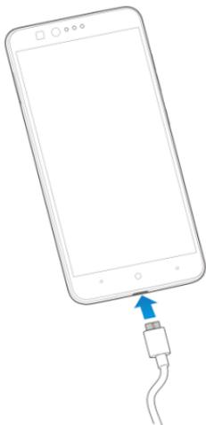
2. Connect the charger to a standard AC power outlet. If the phone is on, you'll see a charging icon, such as
