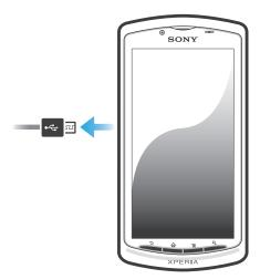
Make sure not to bend the connector when removing the cable from the phone.
