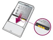
Insert the battery with the battery usage labels facing down and the connectors facing each other.
