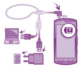
To charge the phone using the power adapter
