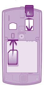
Remove the battery cover, then insert the SIM card and the memory card in the relevant slots.
