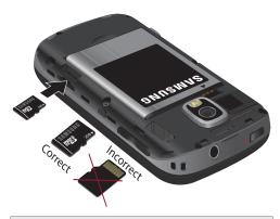
WARNING: Do not over-insert the card as this can damage the contact pins.
