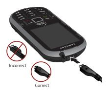
With the Virgin Mobile-approved Li-lon battery, you can recharge the battery before it completely runs down.
