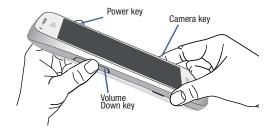
When the device vibrates, release the Power key, but continue pressing the Camera and Volume down keys. Once the device displays the **Are you sure you want to format?** screen, release the Camera and Volume down keys.
