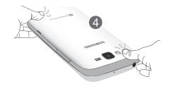
**Note:** Make sure the battery is properly installed before switching on the phone.
