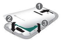
Press down firmly along the edges of the cover to ensure that the cover is flush with the phone (4). You should hear a light click as the cover locks in place.
