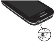
Note: Your phone's internal antenna is located along the bottom back of the phone. Do not block the antenna; doing so may affect call quality or cause the phone to operate at a higher power level than is necessary.
