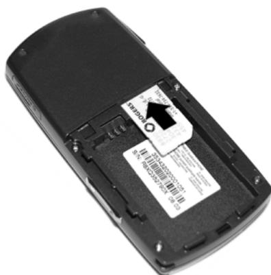
To remove the SIM card, slide it out of the socket.
