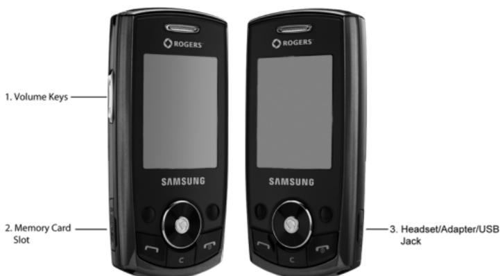
1. **Volume keys/Menu Navigation:** Allow you to adjust the ringer volume in standby mode, mute the ringer when receiving a call and adjust the voice volume during a call. Can also be used to move to the top or bottom of a menu screen.
