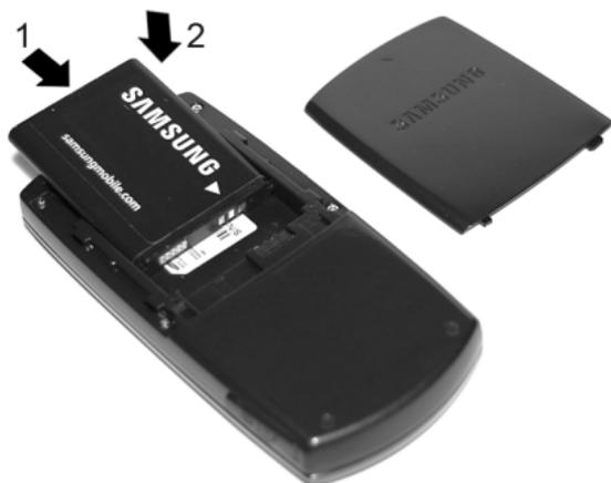
3. With the battery in position in the phone, slide the cover back on the phone until it locks into position.
