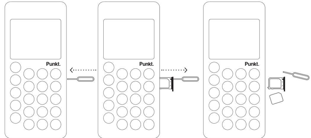
1. Insert the SIM tray pin into the hole on your phone, until the SIM tray pops out.
