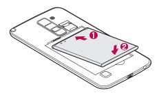
4 To replace the cover onto the device, align the back cover over the battery compartment and press it down until it clicks into place.
