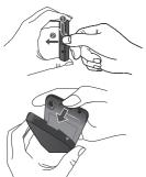
Hold the top edge of the battery and lift it away from the battery compartment.
