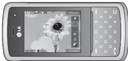
**Note:** You can adjust the zoom using the volume key on the left side of the phone. The zoom function is only available when the resolution is set to 640 x 480 or below. See **Changing the image size** on page 36 for details.
