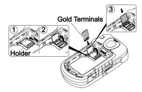
5. Gently press the card and the card holder (4), and then slide the holder in the direction of the arrow to lock it (5).
