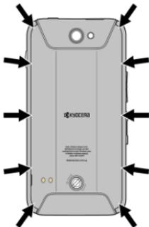
**Warning:** Press all around the edges of the battery door ensuring it is properly sealed to maintain the phone's waterproof capability.
