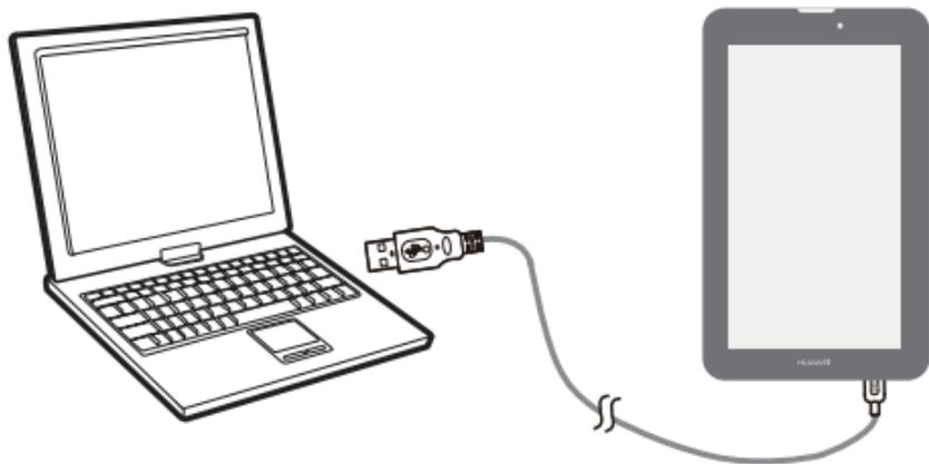
To use USB tethering, ensure that HUAWEI MediaPad has Internet access.
