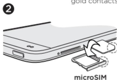
2. Pull the microSIM card tray out. Place your microSIM (contacts facing down and cut-off corner facing out) onto the tray, and then insert the tray back into the slot.
