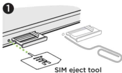
1. Insert the tip of the SIM eject tool (or a small bent paperclip) into the small hole next to the microSIM card tray, and push it all the way in until the tray ejects.
