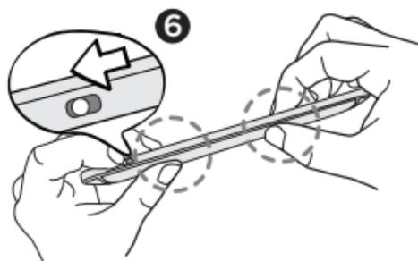
6. Press again on the right side to secure the cover into place, and then slide the lock all the way to the closed position.
