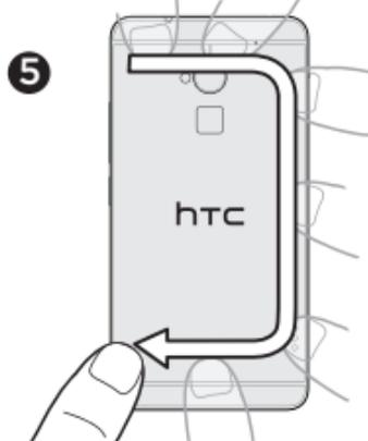
1. Slide the back cover lock, and then lift the back cover from the side.
