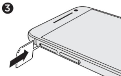
3. Use the same tray eject tool to eject the microSD™ card tray. Pull the tray out.
