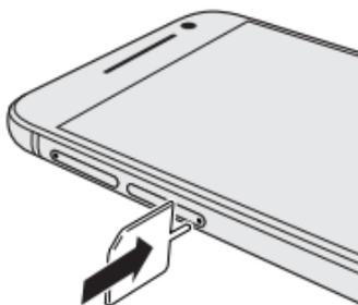
1. With the phone facing *up*, insert the tip of the tray eject tool that came with your phone (or a small bent paperclip) into the hole on the nano SIM slot.
