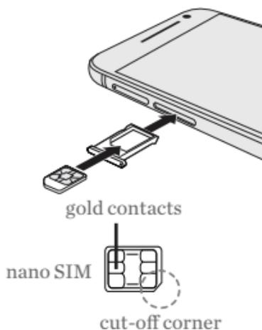
2. Place your nano SIM card into the tray, with the gold contacts facing *up* and cut-off corner facing *out*.
