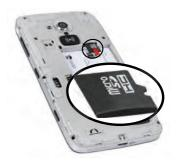
**Tip:** Take care not to scratch or bend the contacts on the memory or SIM card when inserting them into the card holders.
