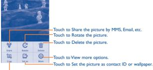
Touch to Crop the picture. Drag the four sides of the rectangle that appears in or out to set the desired cropping size, then touch **Save** to save as a new picture.
