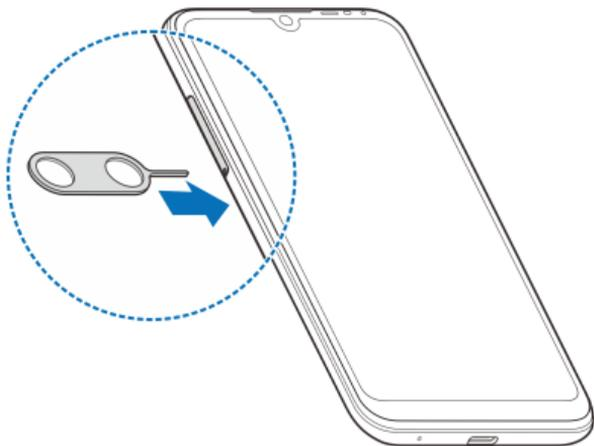
2. Pull out the card tray and place the nano-SIM card and the microSDXC card (optional) on the tray, as shown. Carefully slide the tray back into place.
