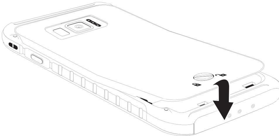
8. Press along the edge of the back cover until you have a secure seal.
