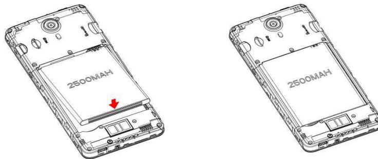
Align the contacts of the battery with the contacts in the phone and gently press the battery down into place.
