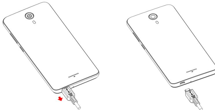
Unplug the AC adapter from the outlet and remove the USB cable from the phone and the AC adapter.
