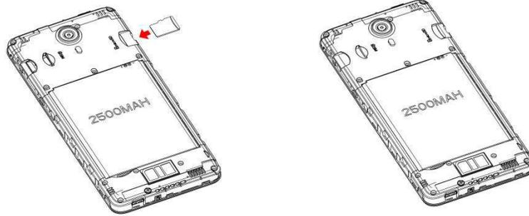
Insert SD card all the way gently without bending and with terminals facing down.
