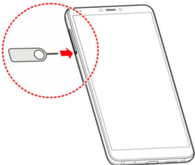
2. Pull out the card tray. You can place a nano-SIM card on the right card slot, and place a microSD card on the left card slot, as shown. Carefully slide the tray back into place.
