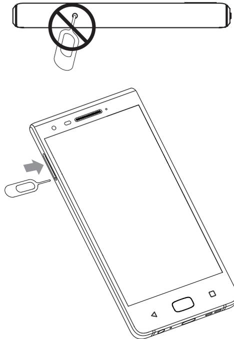
2. Pull out the SIM/microSD tray completely and set it on a flat surface.
