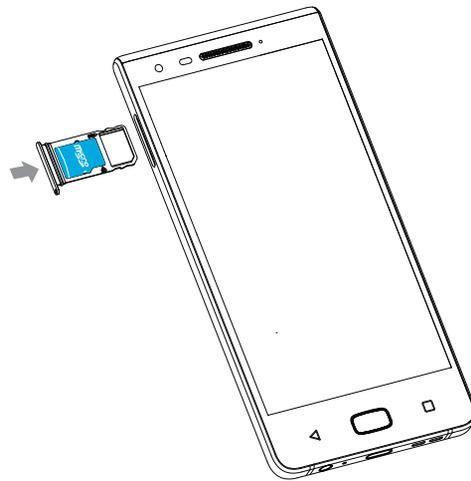
5. Push the SIM/microSD tray back into the slot.
