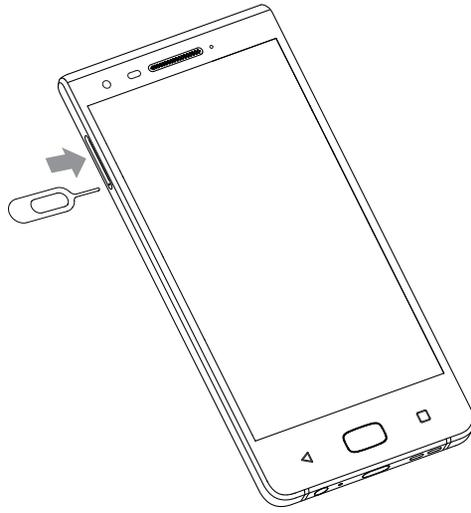
2. Pull out the SIM/microSD tray completely and set it on a flat surface.
