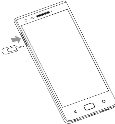
3. Pull out the SIM/microSD tray completely and remove the media card.
