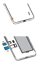
With the phone face down, remove the back cover by gently pulling up on the indentation on the bottom left of the cover.
