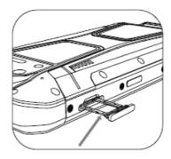
**3** Place the metal side of the Nano card face down, at an oblique angle to the bevel of the card, and place it in the card slot as indicated by the arrow in the illustration.
