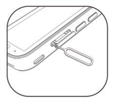
**3** Place the metal side of the Nano card or the Micro SD card face down, at an oblique angle to the bevel of the card, and place it in the card slot as indicated by the arrow in the illustration.
