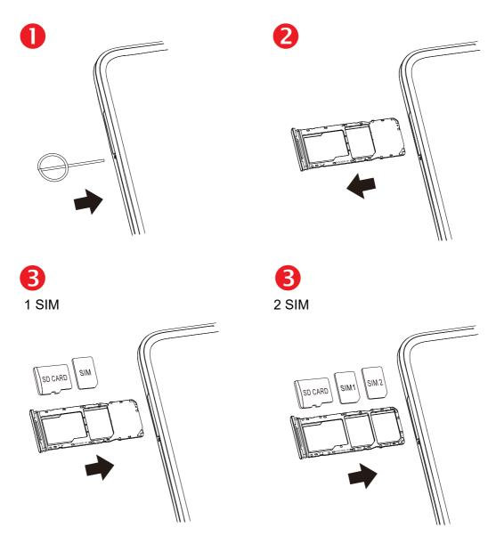
You must insert your SIM card to make phone calls. You do not need to power off your phone before inserting or removing the SIM card as this phone supports hot swap.
