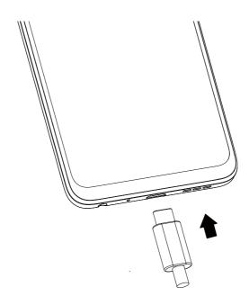
You are advised to fully charge the battery ( ). Charging status is indicated by a percentage displayed on screen while the phone is powered off. The percentage increases as the phone is charged.
