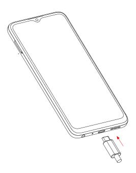
You are advised to fully charge the battery ( ). Charging status is indicated by a percentage displayed on screen while the phone is powered off. The percentage increases as the phone is charged.
