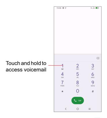
Enter the desired number from the dial pad and touch to place the call or select a contact from **Contacts** or **Call logs** by sliding or touching tabs, then make the call.
