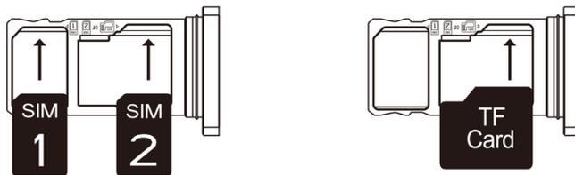
**4** Put the mobile phone face up, and load the card tray with the card 1/card 2 installed into the mobile phone.
