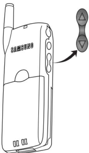
**4. Volume/Scroll Key:** This key is actually two keys (one up and one down) that are used to set the ringer volume, set audio volume levels, navigate through the menus, and change menu settings. Press the volume/scroll key to:
