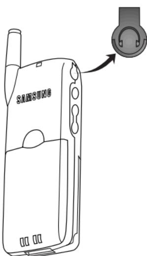
2. **Headset Connector:** This is where you connect the optional headset. The headset includes an earpiece and microphone in a convenient, lightweight unit so you can converse without using your hands.
